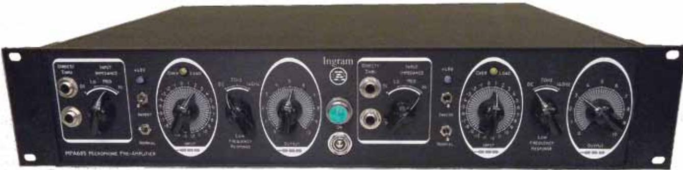
**I**ngram Engineering's MPA685 dual-channel microphone preamp is a large, two-rack-space (14 inches deep) unit that's handmade in the U.S. and features three switchable input-impedance choices and up to 76 dB of gain. Changing the input impedance presented to a microphone by the preamp alters the mic's sound and operation. For the recording engineer, having this ability expands the range of sounds possible from any microphone.
